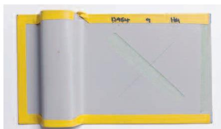
Figure 22. Test panel after Watersoak 1000 hours
