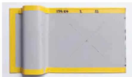
Figure 20. Test panel after prohesion 1000 hours
