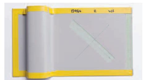
Colorcoat HPS200 Ultra® showed minimal (less than 3mm) edge and scribe delamination following repeated cycles of testing.
