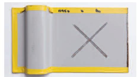
Figure 21. Test panel after humidity 1000 hours
